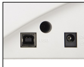
USB port automates plug and play installation.
